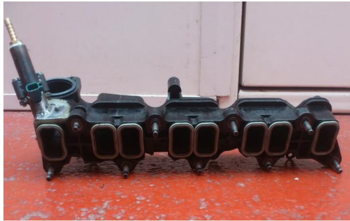
Figure 3.13 Intake Manifold with PFI Injector Installed.
