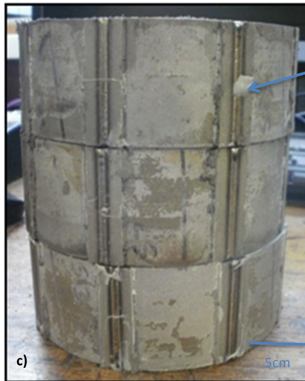
Figure 18 - Photographs of the commercial assembly a) before b) Half the magnets were scored and half were left un-scored c) after hydrogen decrepitation
