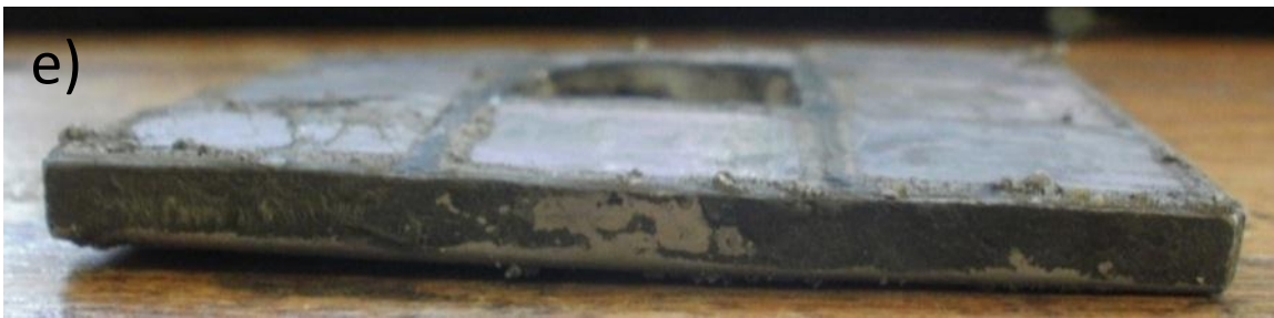
Figure 31 - Mock flate plate assembly after hydrogen decrepitation. a) Entire assembly with line drawn on to indicate bend b) damaged magnet c) damaged magnet d) Uncoated magnet removed by hydrogen decrepitation e) Side view of assembly (the thickness of the plate was 0.8 cm).
