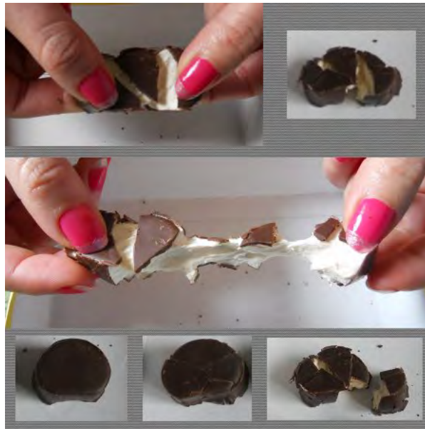
FIGURE 1.1: Different stages in the deformation of a marshmallow covered with chocolate as it is increasingly stretched and allowed to recover its original shape. Top: The marshmallow is stretched beyond its elastic threshold and then photographed as it still tries to recover its original shape. Middle: The marshmallow is stretched beyond its fracture point and it begins to tear at an unpredictable point (the intention was to fracture it at the middle, but only the lower corner got separated). Bottom: Original marshmallow; marshmallow after being pulled on the elastic domain, the chocolate is already fractured, but the marshmallow got fully recovered; marshmallow after the photo in the middle, one corner got separated, but the rest of it almost recovered its shape!
