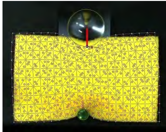
FIGURE 8.5: The deformable target is represented internally as a mesh. Here the mesh is overlapped with the ground truth.
