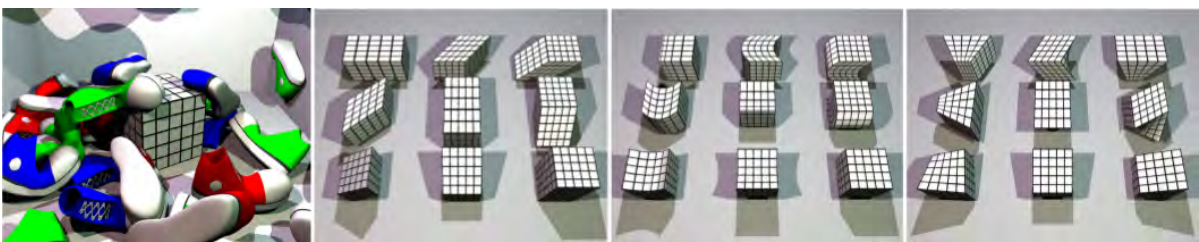
FIGURE 7.8: Shape matching with geometrically inspired modes. The linear shear and stretch modes and the quadratic bend and twist modes are shown. Taken from [56], with permission.
