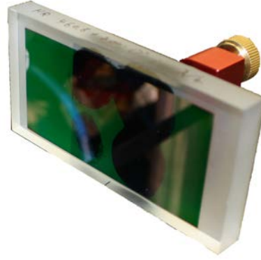
FIGURE 4.20: Photograph of rectangular mirror for the 2D-MOT with foil laminated onto it.
