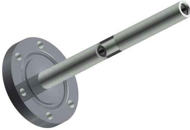
FIGURE 4.5: CAD rendering of Differential Pumping Stage. Carbon tubes are visible on the inside.
