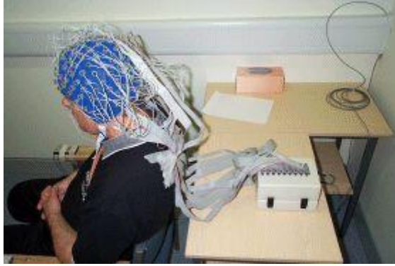
(Sample picture of a participant fitted with an electrode cap and EEG electrodes)
