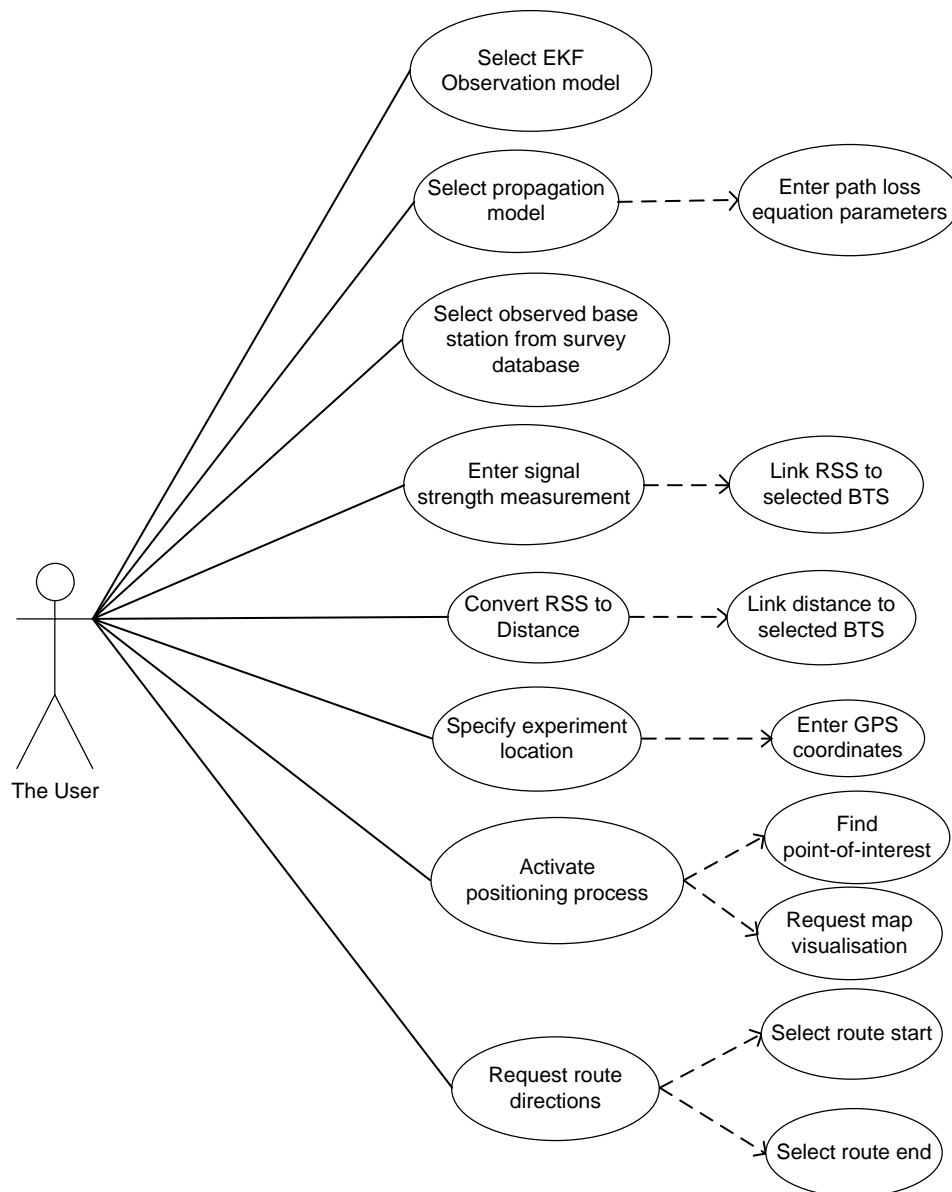
Figure 5.2 GSM Mobile Locator Use Case Diagram
