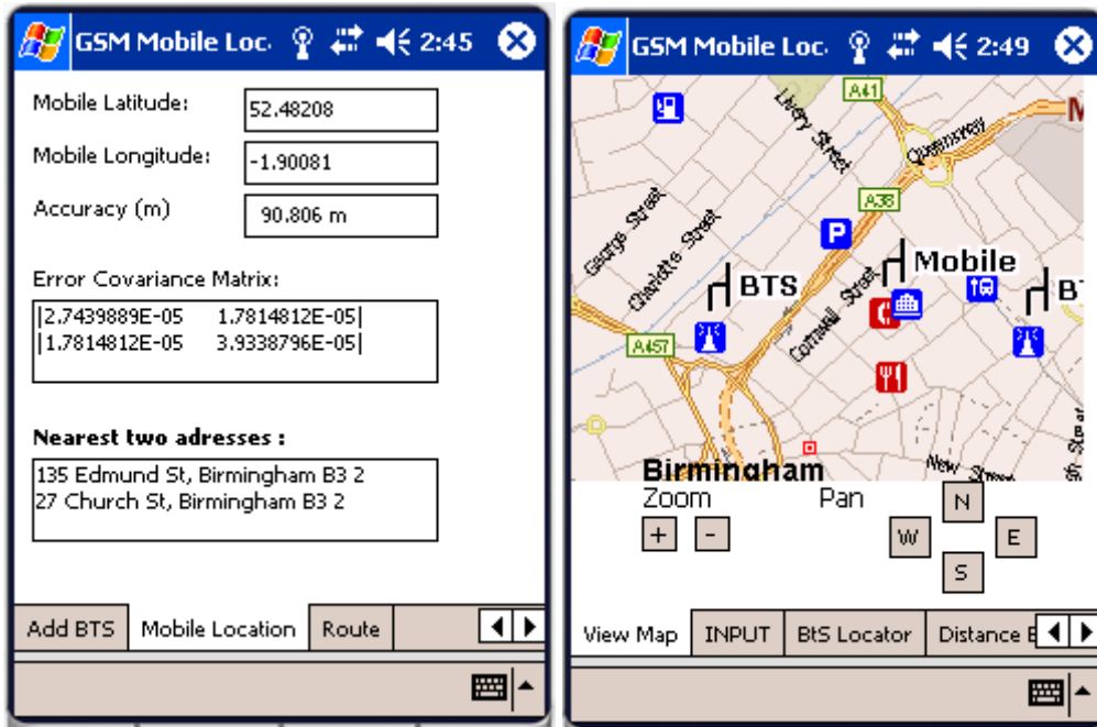
Figure 6.10 The estimated mobile position (GSM Mobile Locator)
