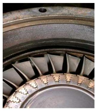
Figure 2 – Blade used in modern turbine engines using single crystal technology.
