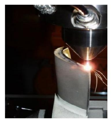
Figure 5 – Illustration of laser repair of blade tip.
