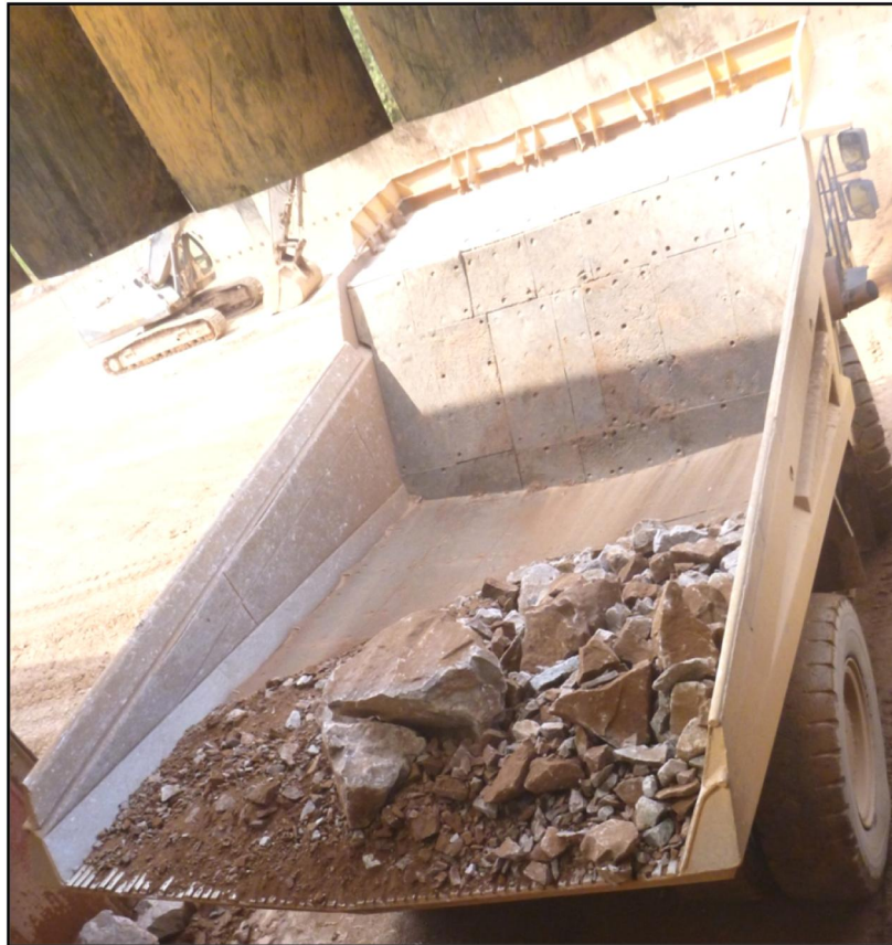
Figure 14: Image of a dumper truck leaving the primary crusher at Mountsorrel Quarry after unloading but still carrying some rock particles.
