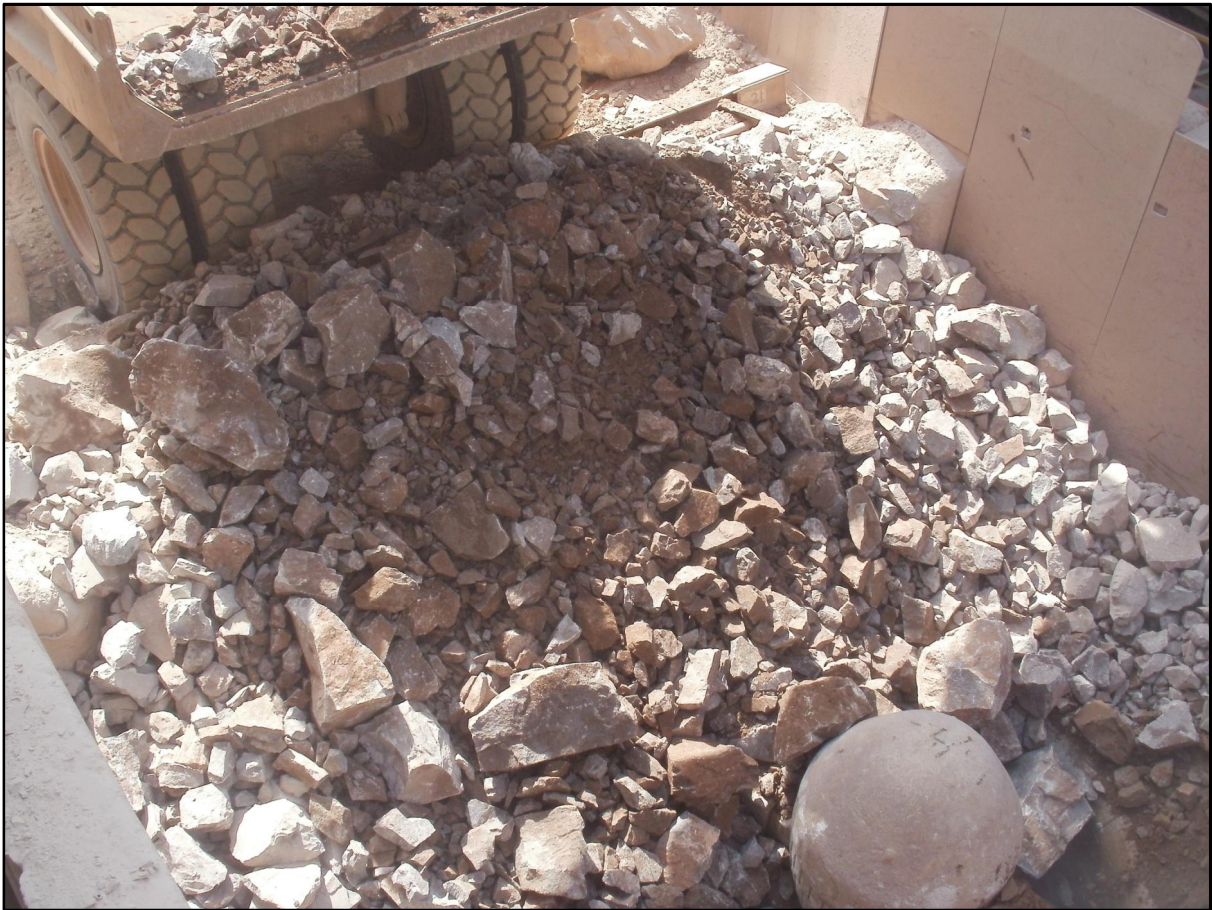
Figure 17: Initial image of a dumper unloading into the primary crusher at Mountsorrel Quarry before being analysed with Split-Desktop to determine the PSD.
