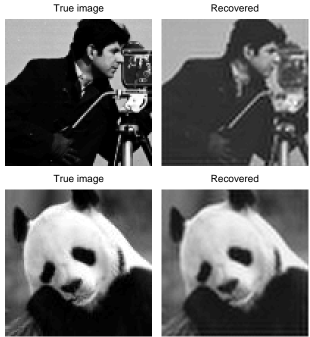
Figure 4.5: Examples image recovery of ‘cameraman’ and ‘panda’ images (10000 pixels) from blurred and down-sampled to 2601 pixels and additive noise with \sigma^2 = 1e-3 using univariate Pearson type VII based MRF.
