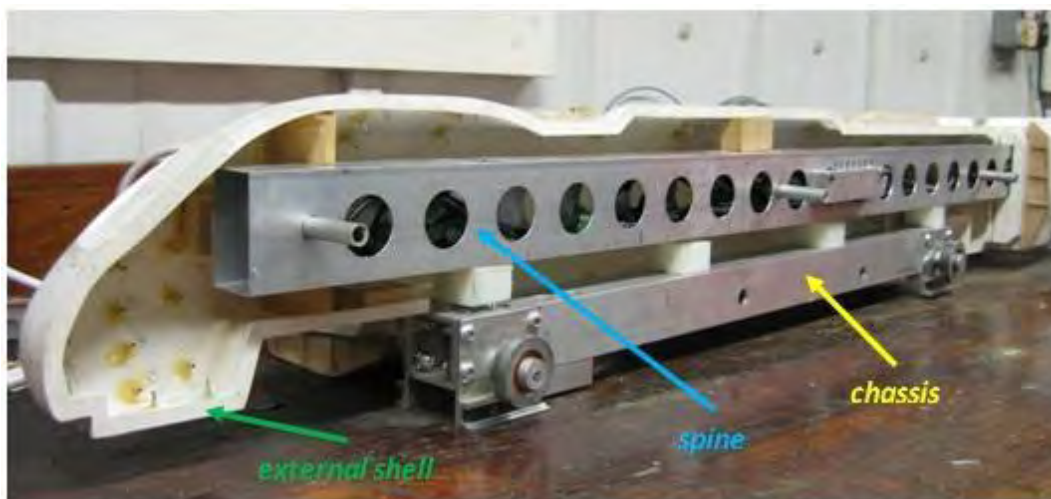
Figure 4.16 Class 390 Pendolino internal model structure
