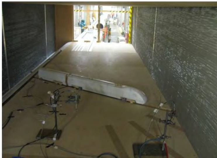
Figure 4.34 View of the Class 390 scale-model inside the CWG during the static tests
