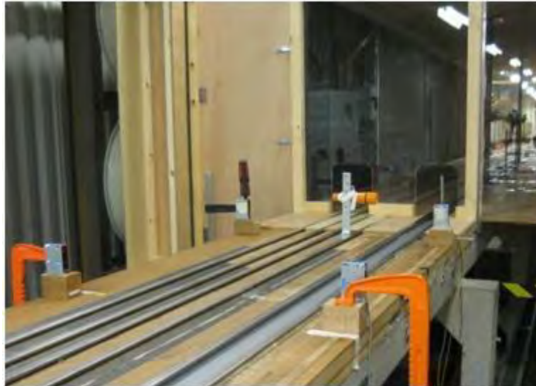
Figure 4.32 Vehicle speed measuring device and trackside light source and light-beam detector
