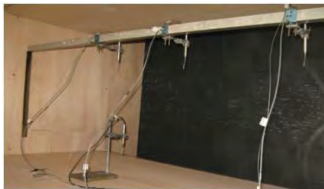
Figure A.15 CWG prototype: flow measurements instrumentation setup
