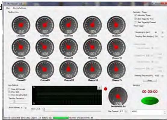
Figure 4.21 On-board data logger a) Control software main panel b) Data output file
