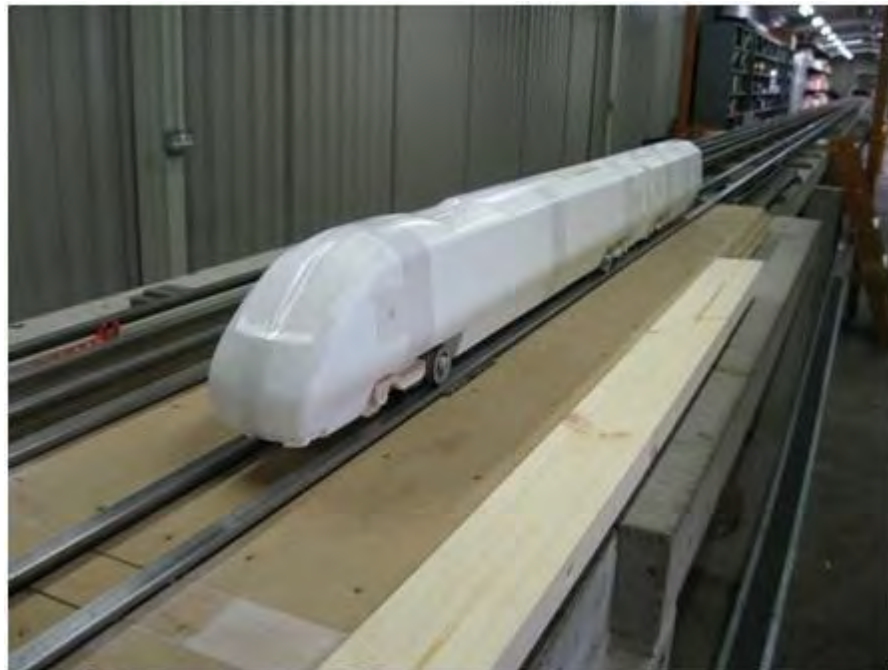
Figure 4.14 Class 390 Pendolino 1:25 scale-model on the TRAIN rig track
