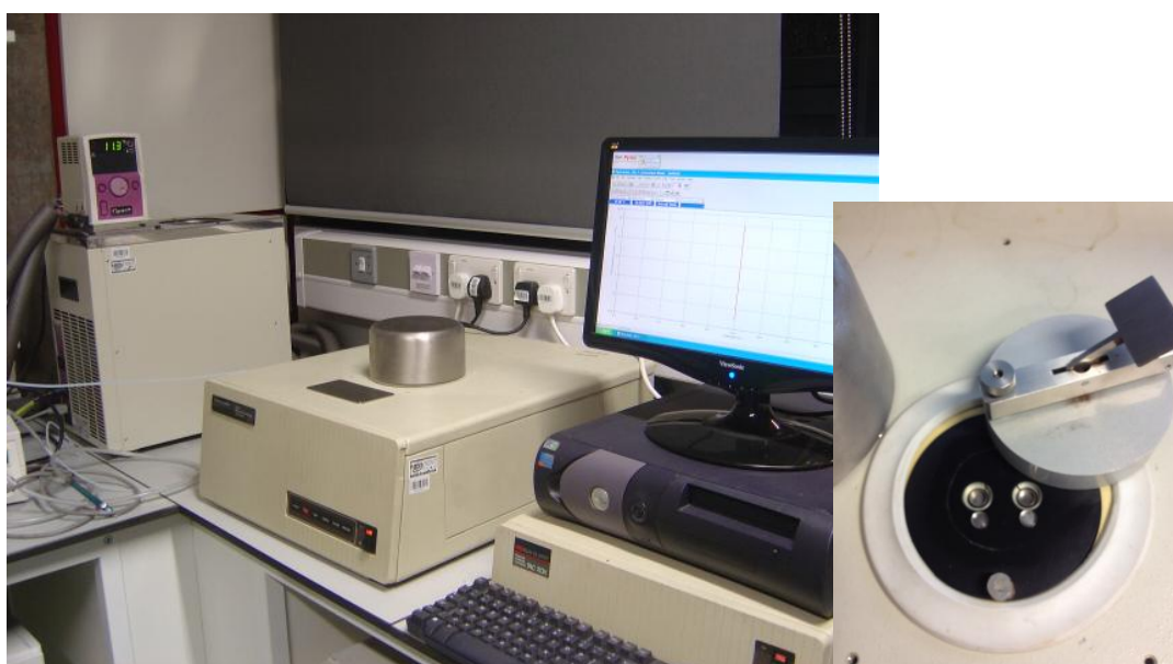
Figure 2.6 The Perkin-Elmer DSC-7 and TAC 7/DZ.
