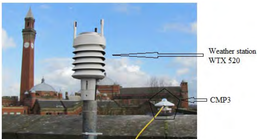
Figure 4-10: Weather station on the roof of the building of School of Civil Engineering. The data logging system relies on radio telemetry which offers a cost-effective, flexible and practical alternative to hard-wired one (Omni Instruments, 2009). The data from a range of sensors located at selected locations in ErgoHome test units are sent to Squirrel receiver logger and this logger transfers all the logging data to a personal computer (PC) by the use of a USB cable.
