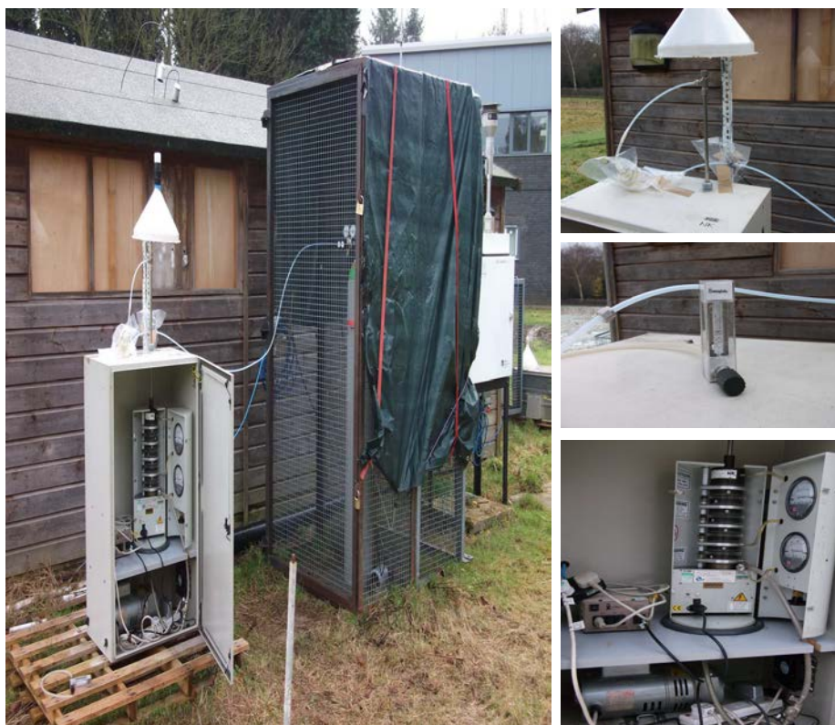
Figure 2.2 Air sampling by the MOUDI with ammonia experiment
