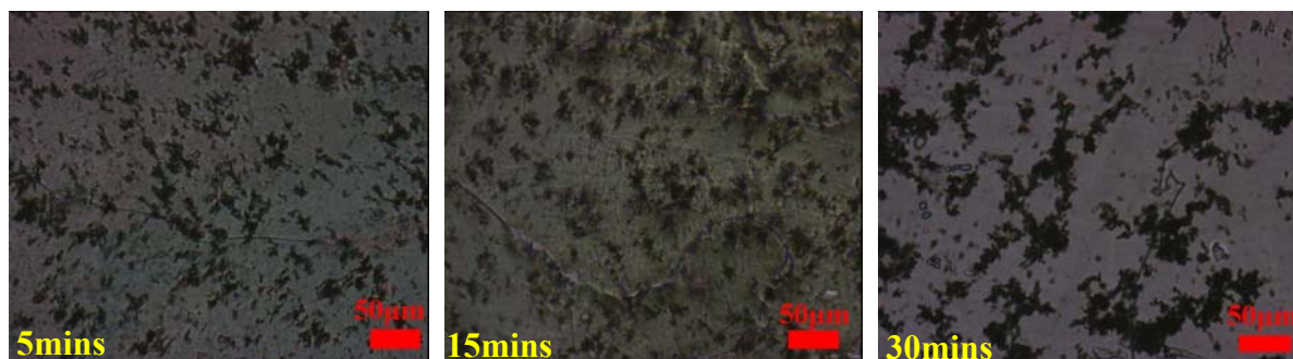
Fig. 3.12 Polarized microscopy images of stirred samples with different sonication time (0.04wt %) at "off" state
