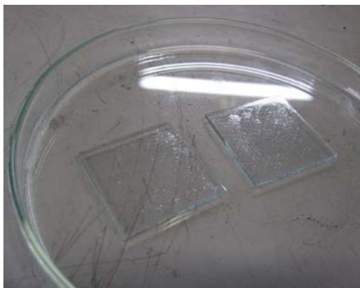
Fig 2.5 ITO glass coated with PVA
