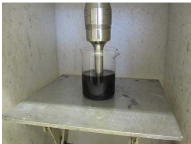
Fig. 2.1 Sonication under 20kHz
