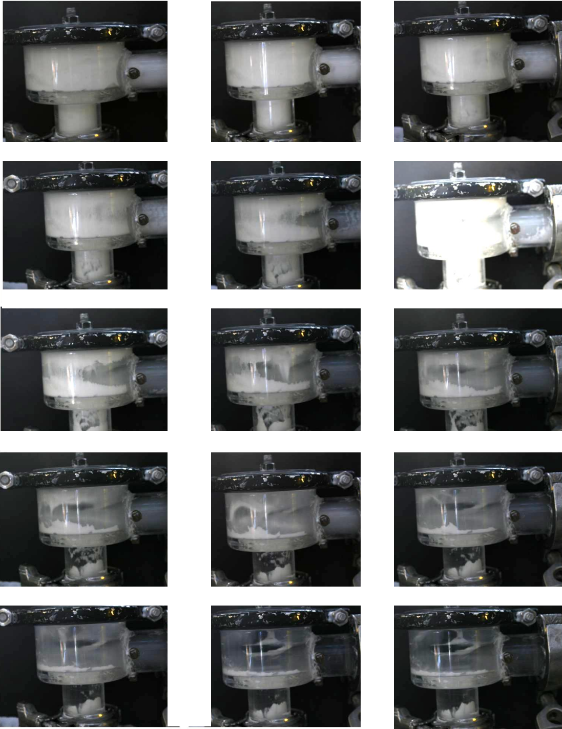
Figure 7.5: ZEAL Pilot Plant: Single seat valve cleaning experiment – using the glass valve especially made for cleaning studies by Bo Jensen . The flow comes from the bottom of the valve and exits from the pipe of the right hand side of the images. Images were taken every second (cleaning condition 20°C, 1 m s -1 based on a clean system inlet of 23.9 mm). Image sequence order, Left to Right, Top to bottom.
