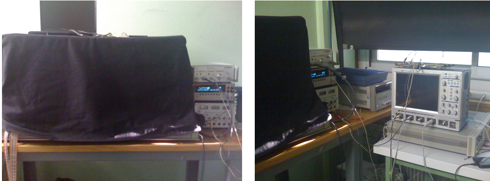
Figure 5.6: Left side: Dark box, Laser control system and HV power supply. Right side: ADC sampling oscilloscope.
