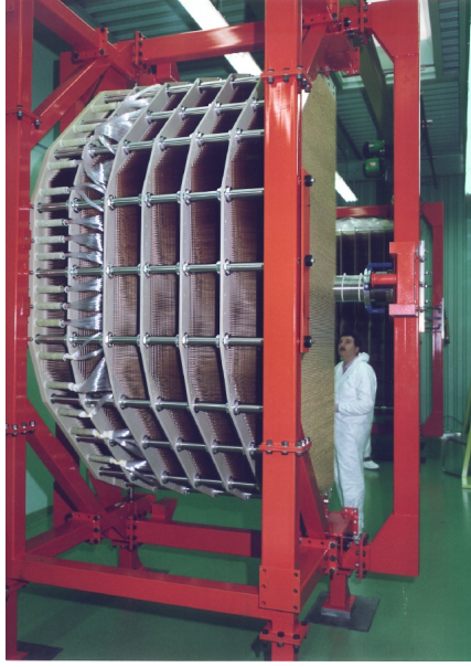
Figure 2.6: LKr calorimeter: (left) half structure while under construction; (right) details of the cell structure.
