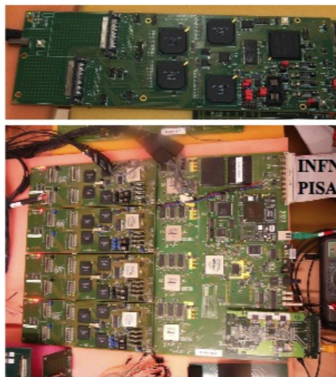
Figure 6.7: CEDAR new front-end and readout system designed for NA62.
