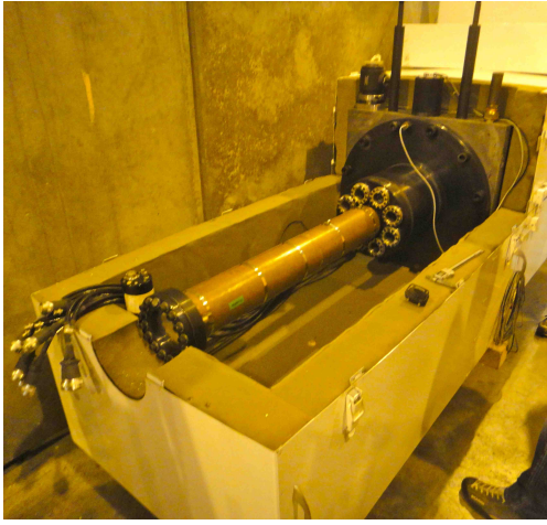
Figure 5.1: CEDAR counter: (left) upstream end view of the vessel with the nose and the quartz windows; (right) schematic layout of a standard West version.
