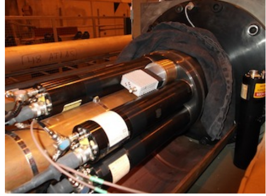
Figure 6.10: Left: the new-PMTs assembly layout and its relative position with respect to the Cherenkov light ring (red circle). Right: CEDAR setup with seven standard PMTs and the new-PMTs assembly.
