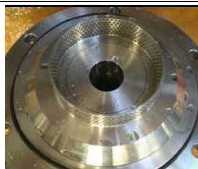
Single standard emulsor stator – used in config. D and G
