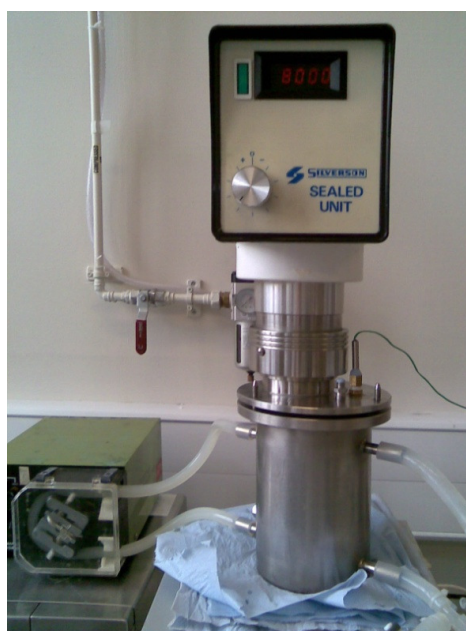
Figure D.1: Batch L4R rotor-stator mixer.
