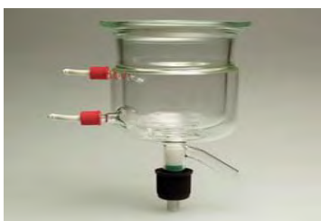
Figure 19 showing jacketed reactor
