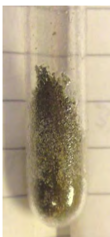
Figure 3.1 The resultant silica tube where a reaction mixture was heated in direct contact with the silica. The smooth surface had been pitted.
