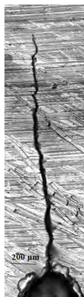
Figure 53 Replica micrograph showing the crack length at 750 cycles
