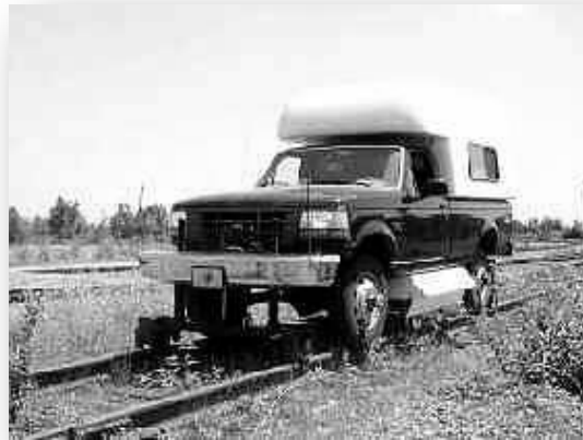
Figure 5 EMAT inspection system for automated rail inspection mounted on a hi-rail vehicle(University of Birmingham, 2007)
