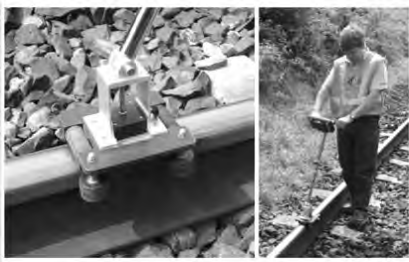
Figure 4 Trolley mounted crack detection method(Hocking NDT Ltd, 2012)
