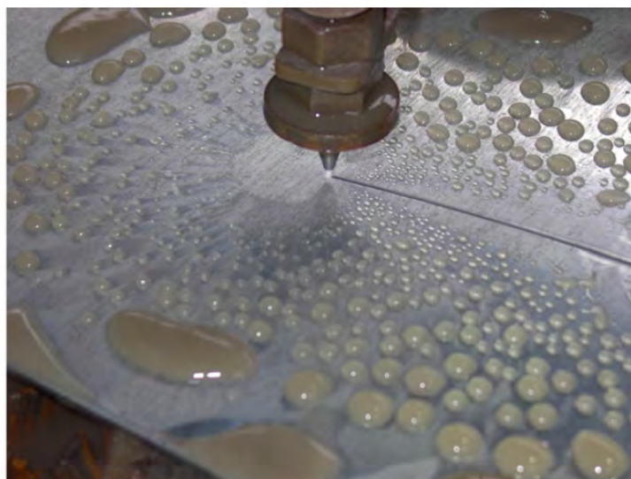
Figure 2.3: A figure showing the cutting of metal plates by high speed water jets. Reproduced from Eggers and Villermaux (2008).
