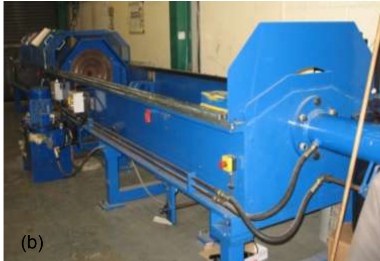
Figure 30(b). Photograph of the mandrel extraction unit used during site trials.
