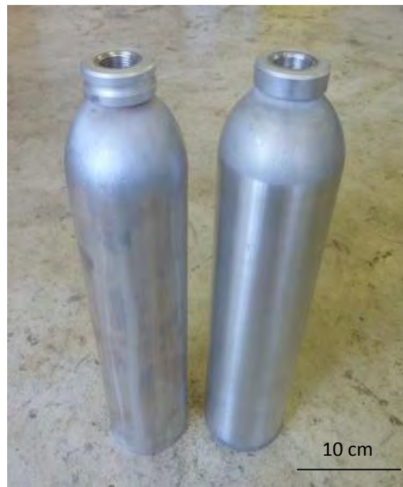
Figure 35. Photograph of aluminium liners used to manufacture composite overwrapped pressure vessels (COPV's).
