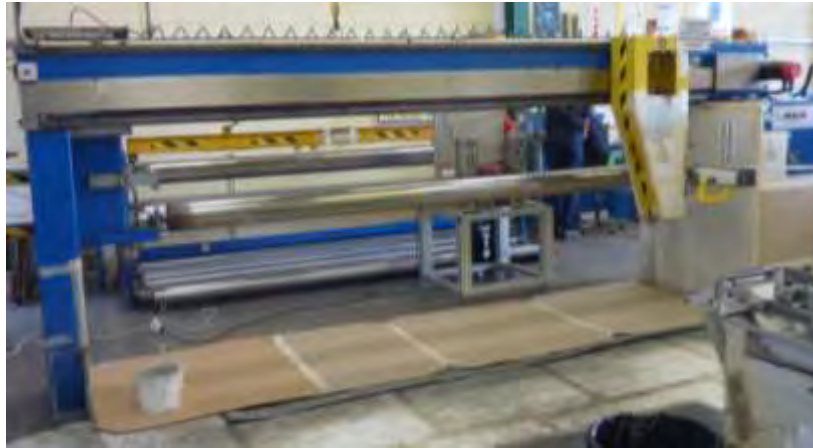
Figure 28. Photograph of the conventional 2-axis filament winding machine used during the industrial site trials in Portsmouth, UK. The scale is indicated by the 3 m mandrel mounted on the machine.
