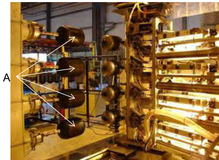
Figure 2. Multi-component filament winding [57]. Here, four carbon fibre pressure vessels (A) are filament wound simultaneously.
