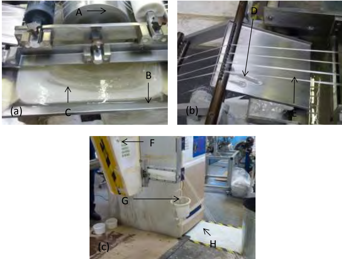
Figure 74. Photographs highlighting the issues associated with conventional filament winding, in particular: (a) the resin bath with obvious air ‘bubbles’ present in the resin; (b) resin dripping onto the conventional guiding equipment; and (c) ‘waste pots’ catching excess resin drips. The highlighted components are: (A) a resin drum; (B) resin bath; (C) resin ‘bubbles’; (D) resin drips; (E) impregnated fibres; (F) traversing arm; (G) plastic container catching resin drips; and (H) protective flooring.
