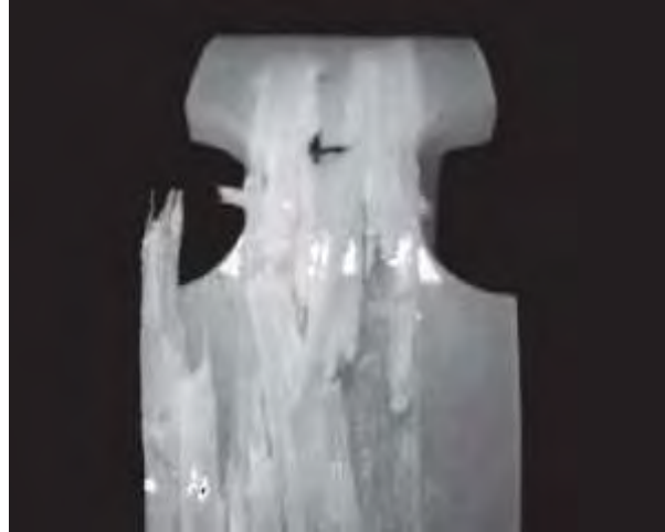
Figure 7. Image of a failed hoop tensile (split-disk) testing sample presented by Sobrinho et al [89].
