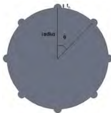
Figure A1. Schematic illustration of a ridged fibre spreading pin [110].
