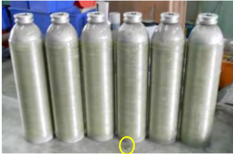
Figure 81. Photograph of the COPVs manufactured with the in-house CFW method. Here, the highlighted scale is a UK £1 coin.
