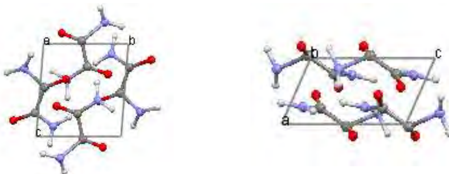
Figure 5.19, The best model structure of oxamide located by direct space structure solution from the biphasic powder pattern recorded for sample 4.
