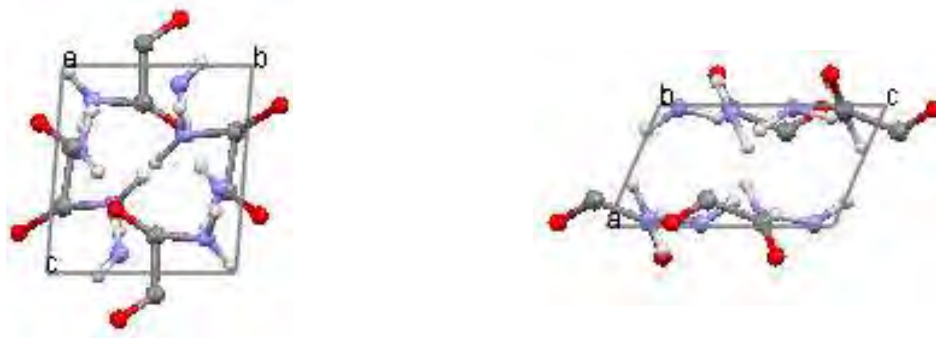
Figure 5.23 , The best model structure of oxamide located by direct space structure solution from the biphasic powder pattern recorded for sample 5.
