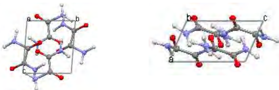
Figure 5.25 , The best model structure of oxamide located by direct space structure solution and simultaneous quantitative phase analysis from the biphasic powder pattern recorded for sample 5.
