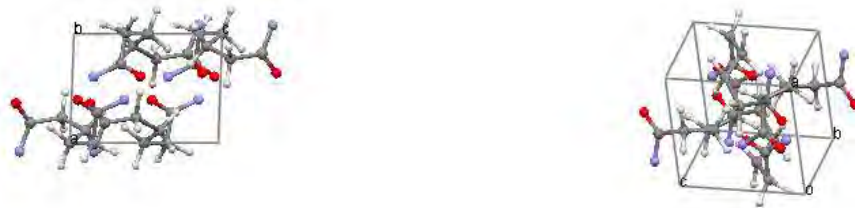
Figure 5.18, The best model structure of adipamide located by direct space structure solution from the biphasic powder pattern recorded for sample 4.
