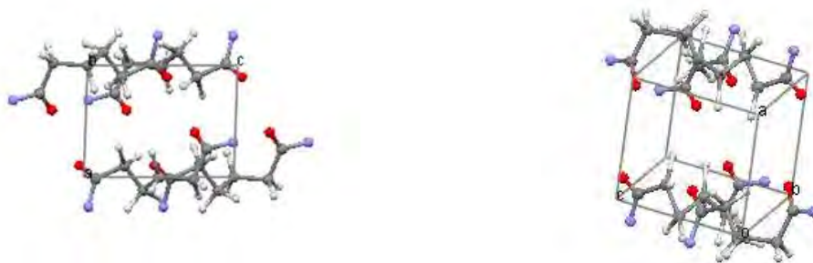
Figure 5.12 , The best structure of adipamide located by direct space structure solution and simultaneous quantitative phase analysis from the biphasic powder pattern recorded for sample 1.
