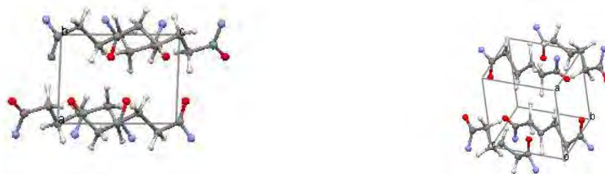
Figure 5.16 , The best model structure of adipamide located by direct space structure solution and simultaneous quantitative phase analysis from the biphasic powder pattern recorded for sample 3.
