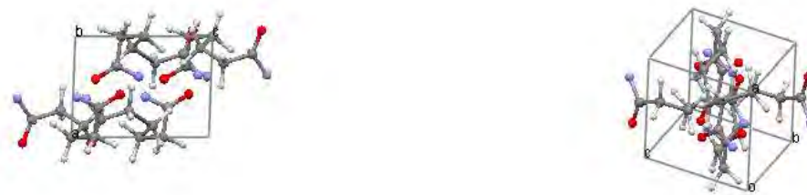
Figure 5.20 , The best model structure of adipamide located by direct space structure solution and simultaneous quantitative phase analysis from the biphasic powder pattern recorded for sample 4.
