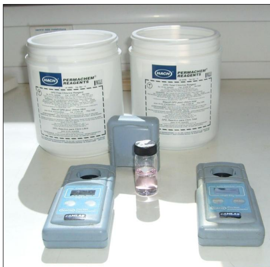
Figure 3-8: Photograph of pocket Hachs chlorine meters and the pink colour produced in the water cells.
