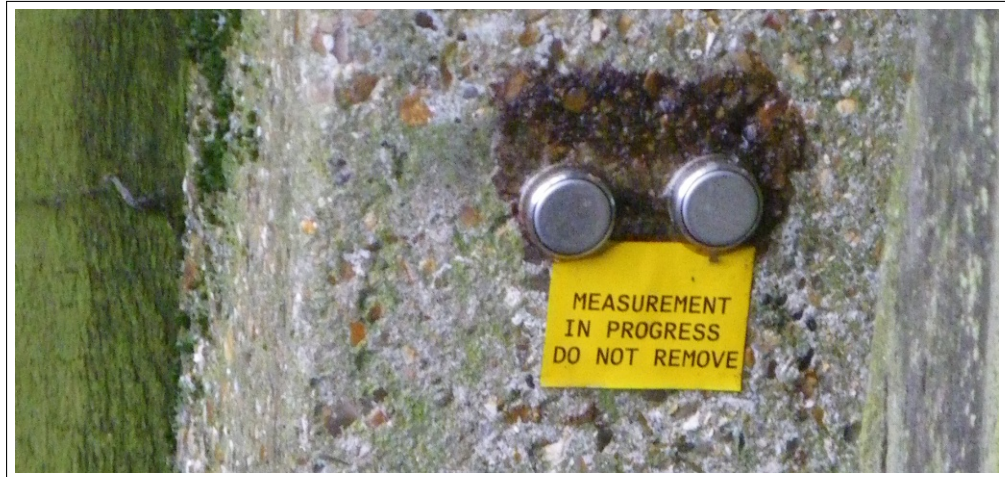
Figure 5.2: Pair of iButton temperature loggers installed.
