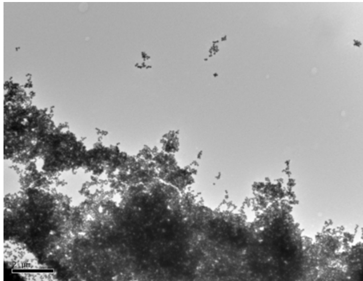
Figure 8.10: TEM image (3) of the spherical hematite particles in 100mM \text{KNO}_3 after 30 minutes at a stirrer speed of 200rpm without a magnetic field.
