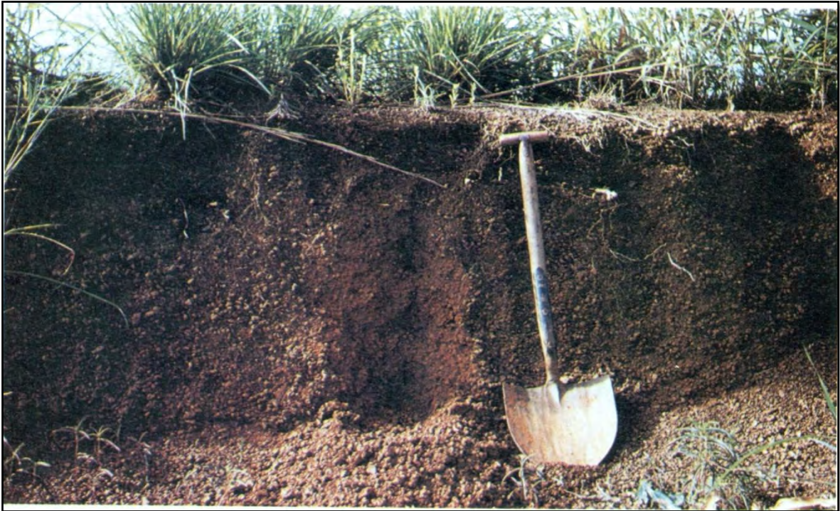
Figure 2.11 - Nodular Lateritic Gravel (Charman, 1988)
