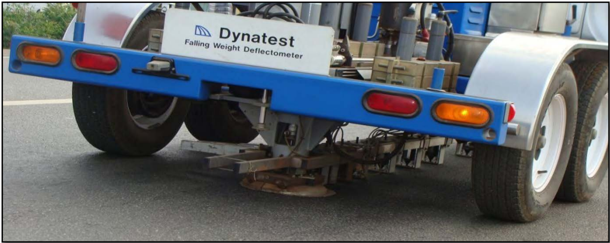
Figure 4.27 – The FWD in Operation
