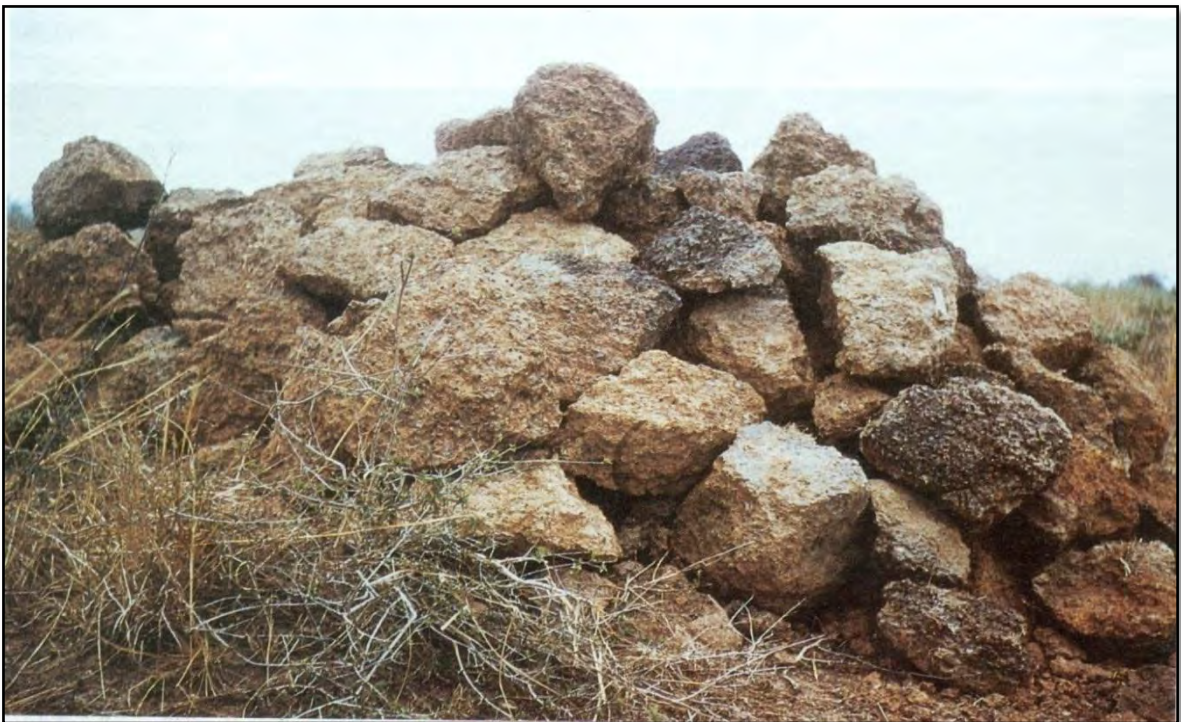
Figure 2.12 - Concretionary Laterite Boulder (Charman, 1988)
