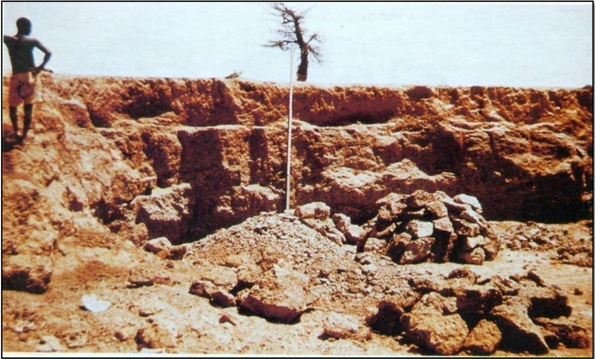
Figure 2.13 - Hard Concretionary Laterite (Charman, 1988)
