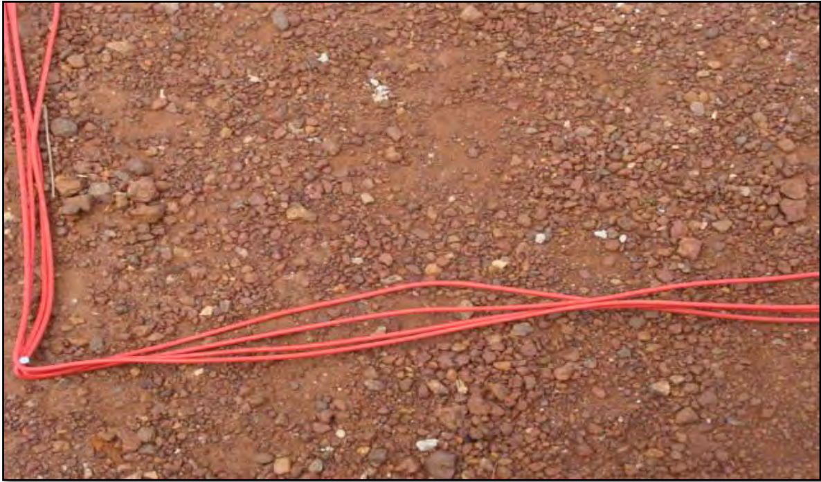
Figure 4.10 – Specified Turns of Induction Loops
