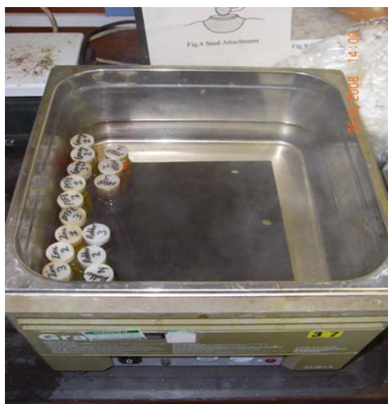
Fig 3.6 Image of MQP samples in water bath setup.
