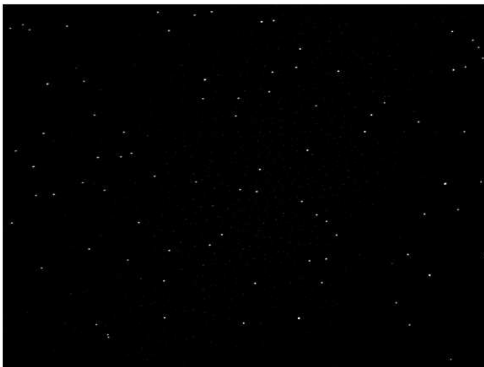
8.8 B: 200x cross polar optical microscopy image of a 0.0001g solution of 0.5 \mu\text{m} silica particles
