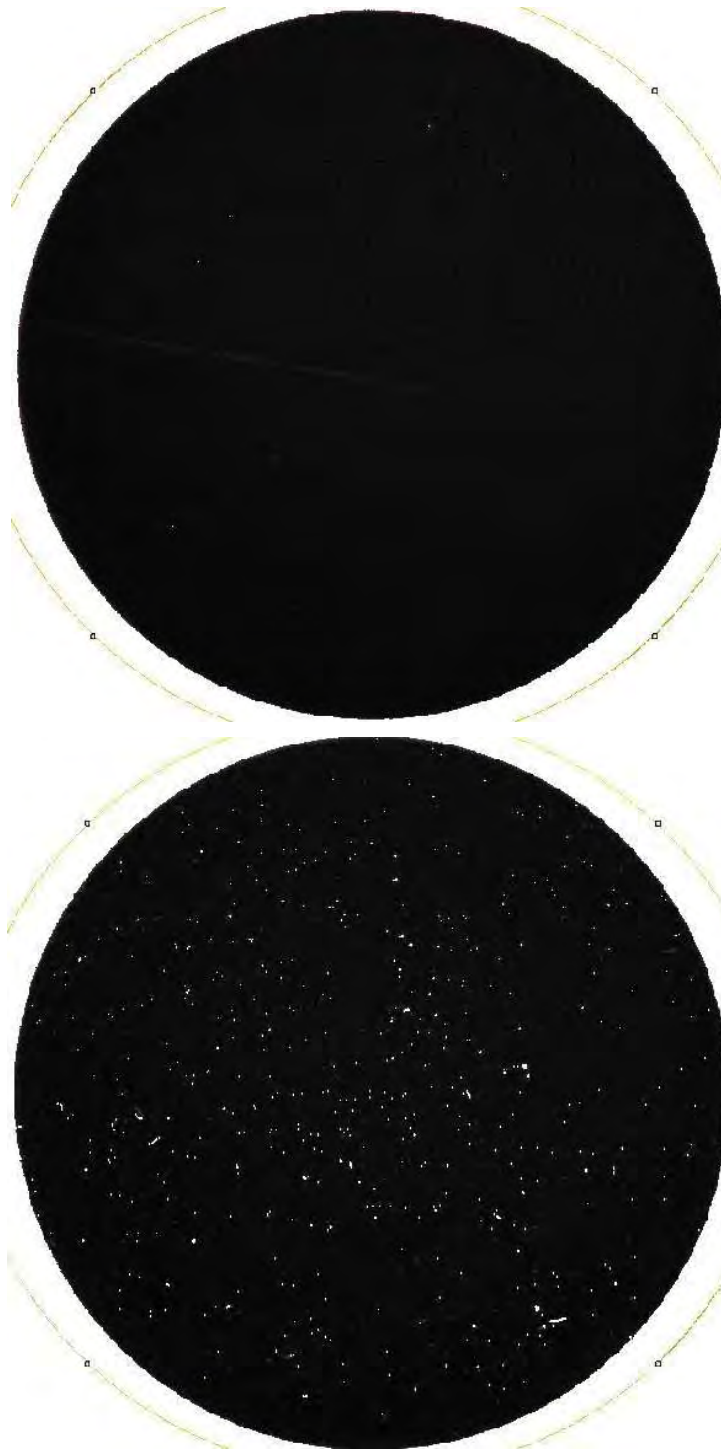
Figure 7.13: Calcium test buttons from samples of 'ultra-clean peelable', showing pinhole counts of 5 on the protected button (top) and 408 on the contaminated (bottom), both are 28 mm in diameter
