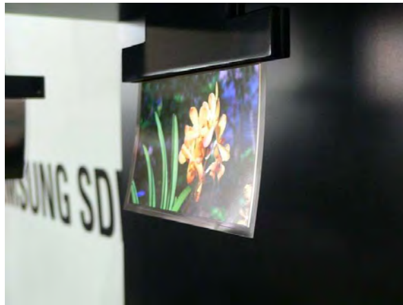
Figure 2.6: Samsung's 0.05 mm thick display panel (Engadget, 2008)
