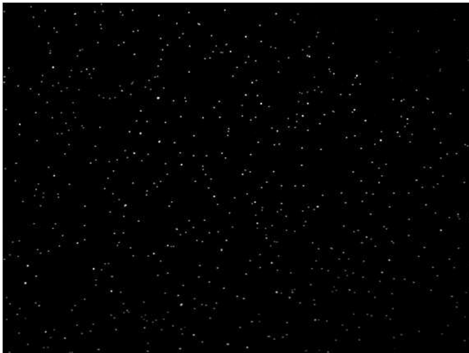
8.8 A: 200x cross polar optical microscopy image of a 0.001g solution of 0.5 \mu\text{m} silica particles
