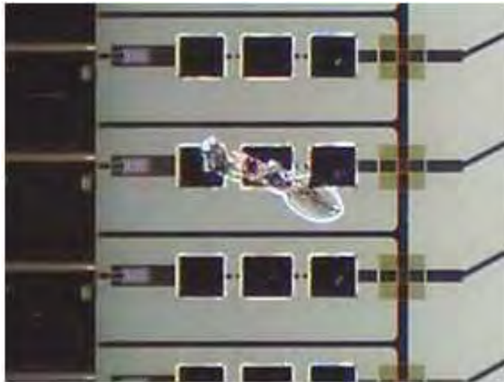
Figure 2.11: Light microscopy image of a short circuit caused in micro-circuitry by a film defect
