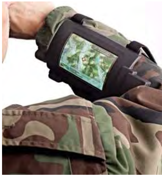
Figure 2.7: 4.3 inch flexible OLED display currently undergoing field testing by the U.S. Army (Engadget, 2010)
