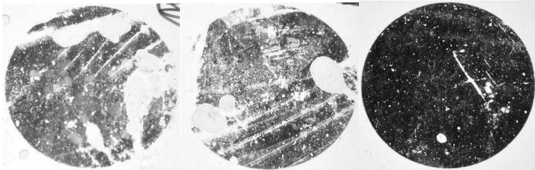
8.19 A: 0.1 µm silica sunken to depths of 25 % (left), 50 % (centre) and 75 % (right) of their total diameters
