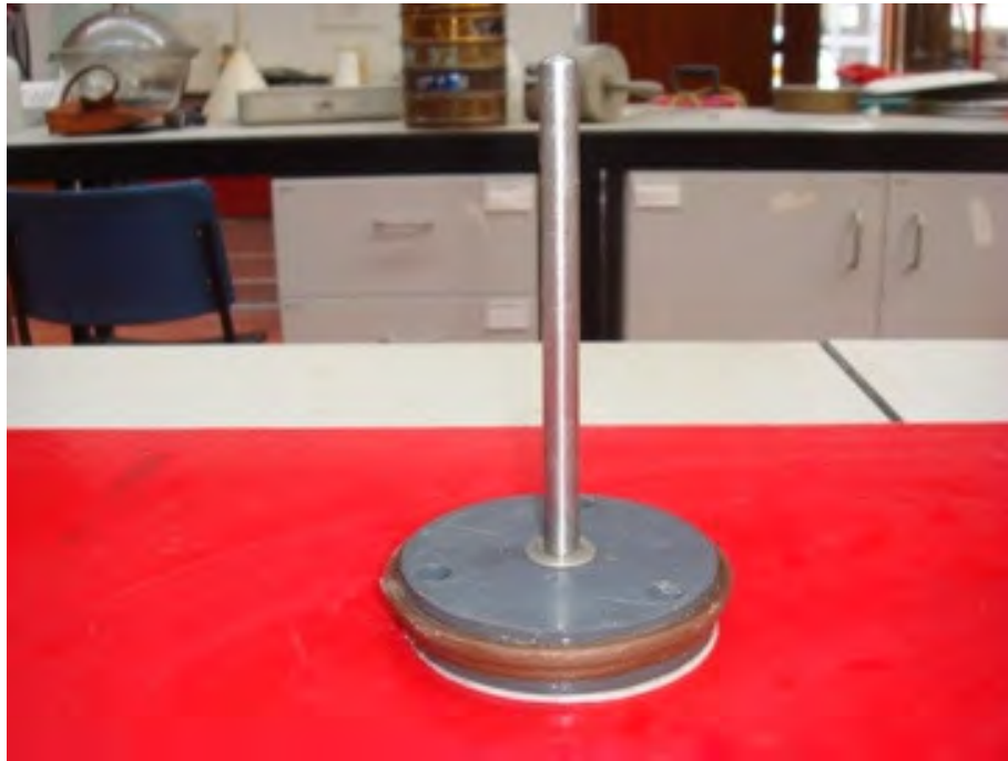
Figure 4.9: Loading plate for EK batch testing to be placed on top of the sample during consolidation.
