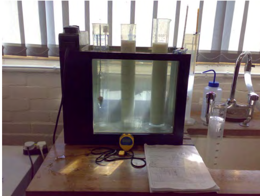
Figure 4.3: Hydrometer test setup
