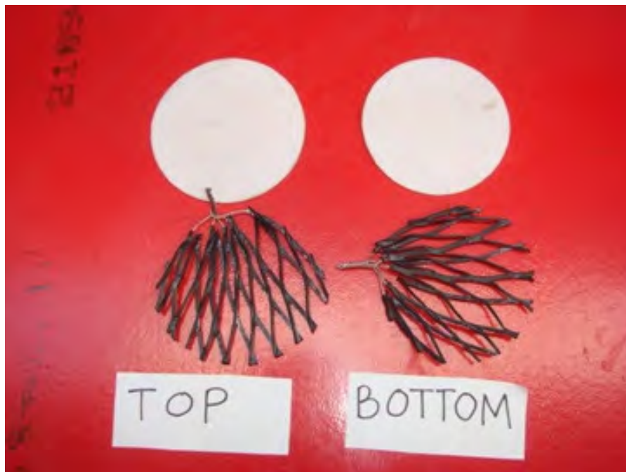
Figure 4.8: EKG electrodes and Vyon sheet filter used in batch testing to be attached at the top and bottom of the sample during electrokinetic treatment.
