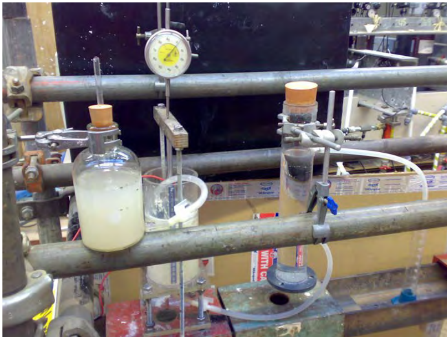
Figure 4.10: Setup and design configuration of EK batch testing.
