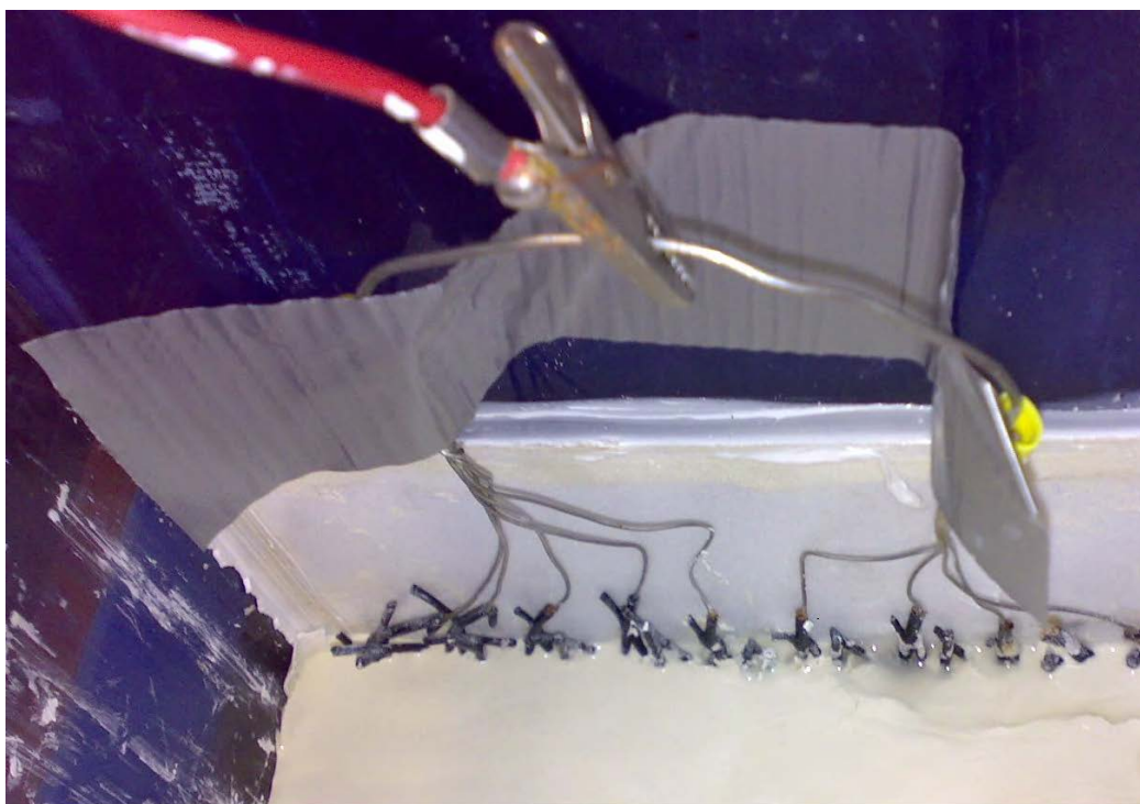
Figure 6.12: Picture of soil electrode interface at the cathode after 3 days during EKS testing.
