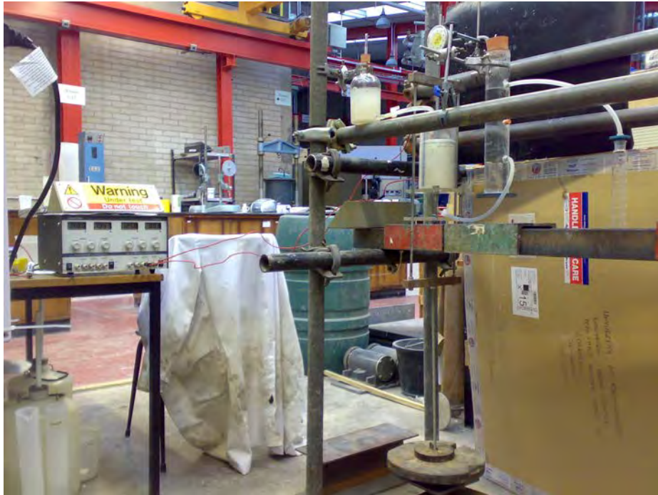
Figure 4.11: Setup of batch testing using the Mariotte bottle method.
