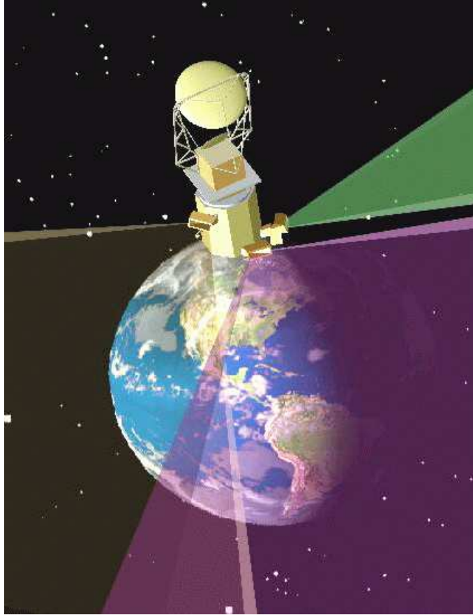
Figure 2.1: An illustration of the SMEI instrument onboard the Coriolis satellite. The three SMEI cameras point away from the Earth and from left to right are Camera 3, Camera 2 and Camera 1, respectively [Webb et al., 2006].
