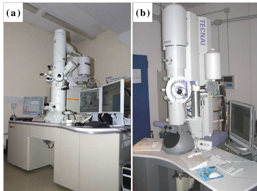
Figure 3.2: images showing a JEM-2100 TEM (a) and a TECHNAI F20 TEM (b).
