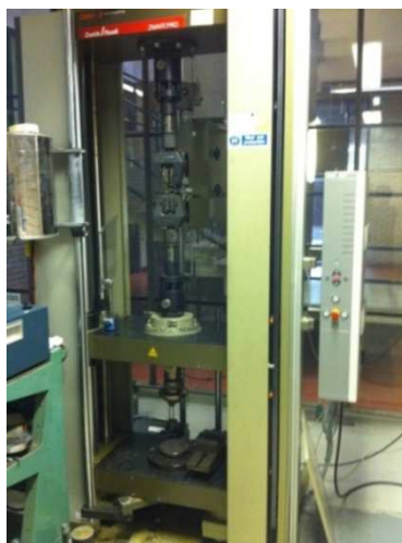
Figure 3.3: image showing the ZWICK-1484 mechanical test machine used in the study.
