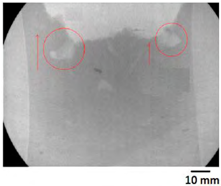
Figure 4-44. The sequences of filling the untreated foam pattern (Probead-30™) in the LFC process.
