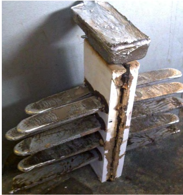
Figure 4-3. One of the fluidity tests, (casting D2)
