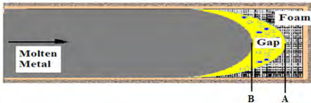
Figure 4-17. The molten metal reached point 14 located at the first level of fluidity strips, cause a sudden increase in the recorded temperature, casting H2.
