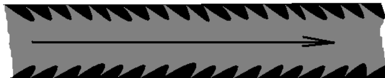
Figure 2-11. Schematic dendritic growth in direction of the flow
