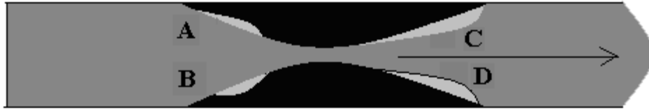
Figure 2-8. Schematic chocking in skin freezing materials.
