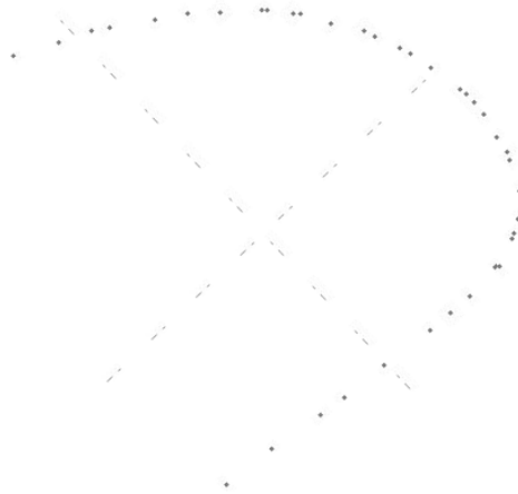
Figure 4: measured aerofoil with a not-constant point density
