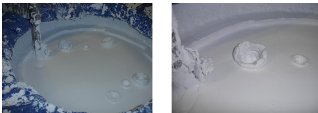
FIGURE 7.1: Images of the original Ludox HSA based SiAl2080 slurry, note the significant flocculation on the surface.
