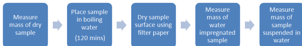
FIGURE 3.14: Measurement process for Archimedes porosity testing of shell specimens.
