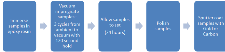
FIGURE 3.17: Process for preparing shell samples for SEM analysis
