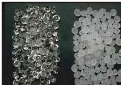
Figure 2.1: Visual appearance of ‘as received’ P D,L LA 3051D Left: Amorphous, transparent pellets; R: opaque, semi-crystalline pellets.
