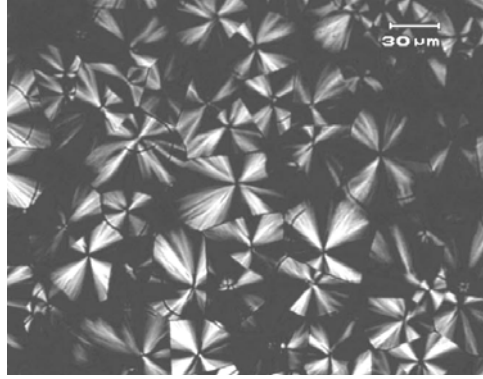
Figure 4.5: Polarised light micrograph of PLLA spherulites showing the ‘Maltese cross’ effect caused by birefringence of polarised light (Permission applied for; Chao et al , 2008).
