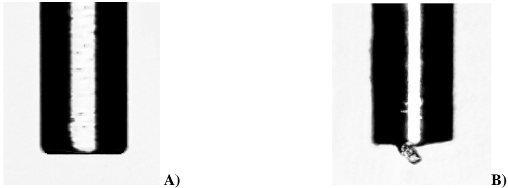
Figure 3.6: Comparison of two different flat ended probes. A) Acceptable flat surface, B) unacceptable end with debris attached.
