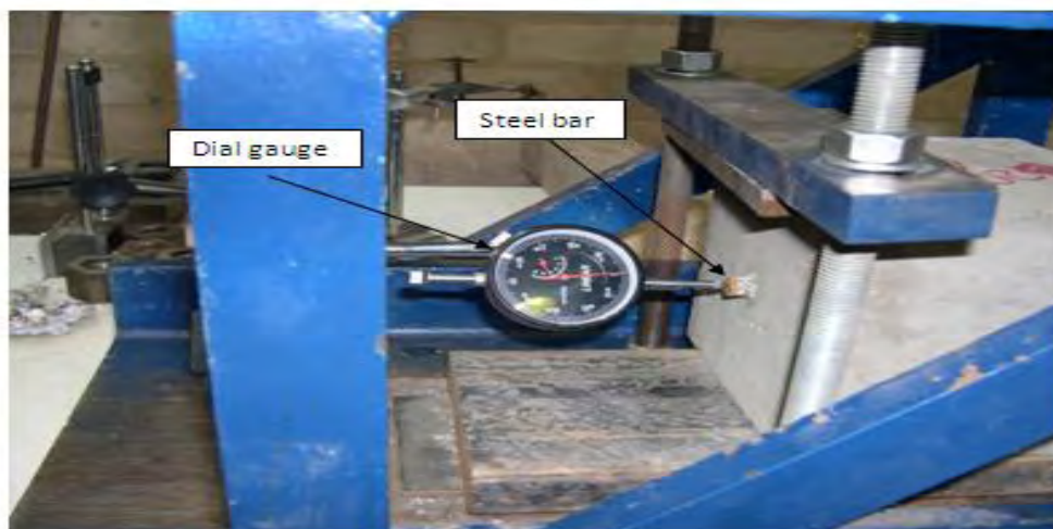
Figure 7-4 Pullout test measurement setup used for bond strength evaluation
