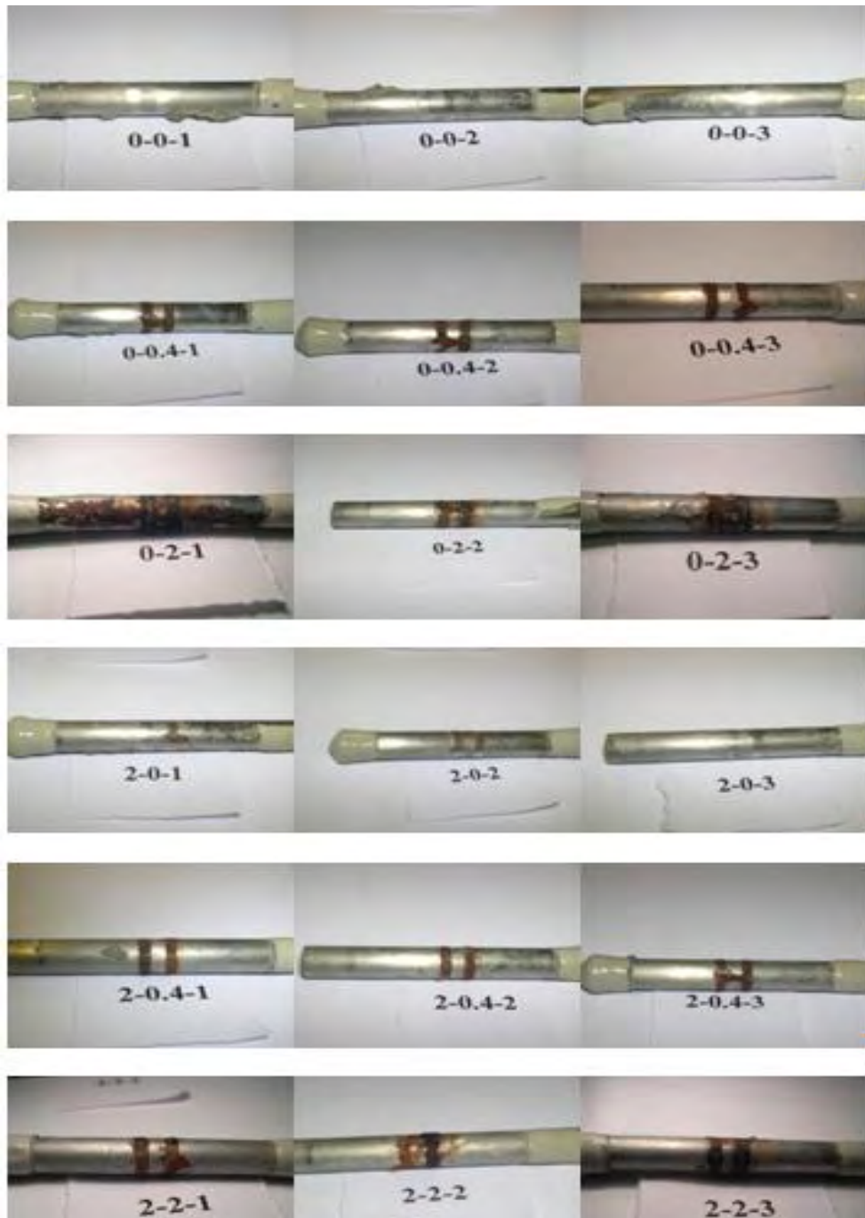
Figure 4-11 The extent of rust in steel bar extracted from mortar containing different levels of chloride and containing 0 and 2 per cent BHD
