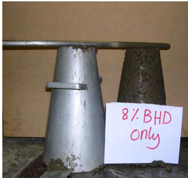
Figure 8-1 Actual concrete slump for 8 per cent addition made without concrete accelerators
