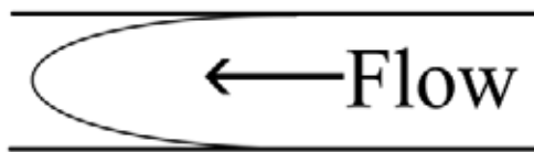
Figure 3.16: The parabolic profile of a laminar flow.
