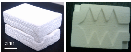
Figure 4: 3D calcium phosphate brackets printed on the 3D powder printing system (Spectrum ZS10, Z-Corporation, USA). Images show two brackets as well as the internal design of a printed bracket.
