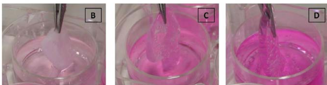
Figure 5.8 Degradation of acellular fibrin gel at 37°C in water, PBS and DMEM (A) and images of self-supporting fibrin structures after 28 days in water (B), PBS (C) and DMEM (D). All gels were formed in 12-well cell culture plates. The error bars shown represent the standard error of the mean.
