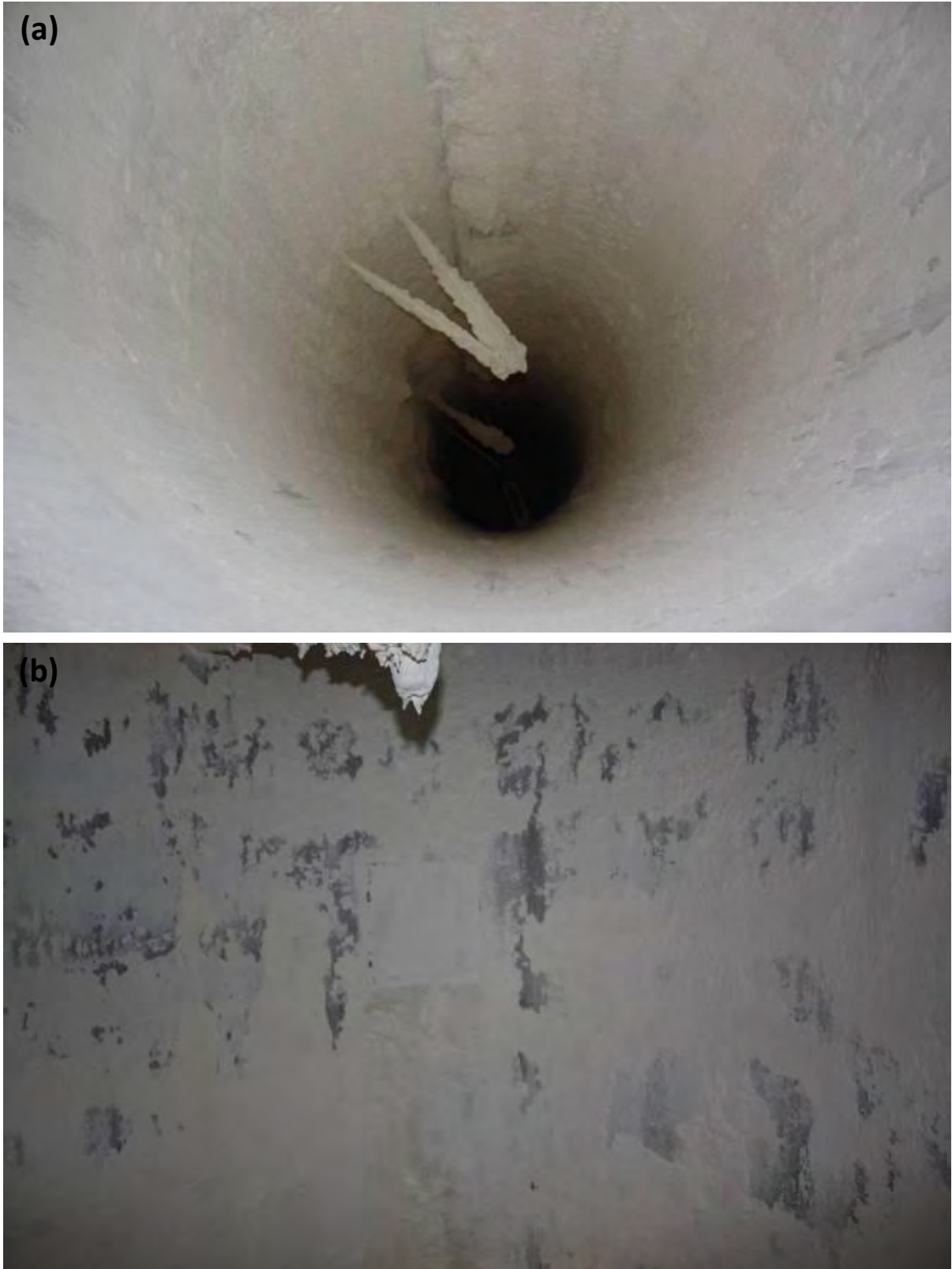
Figure 4.2: Typical wall deposition as viewed from position E: (a) looking down the dryer and (b) close-up of dryer wall
