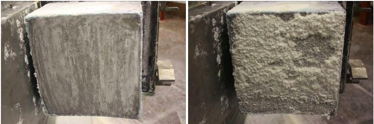
Figure 3.4: Spray Dryer Inspection Hatch Deposition Measurement (before and after operation)
