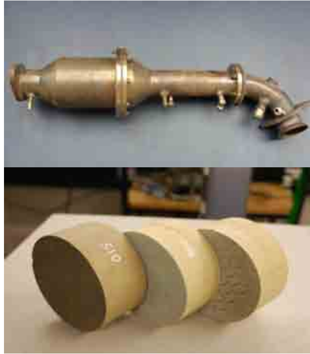
Figure 3.2: Prototype three-zone monolith catalyst
