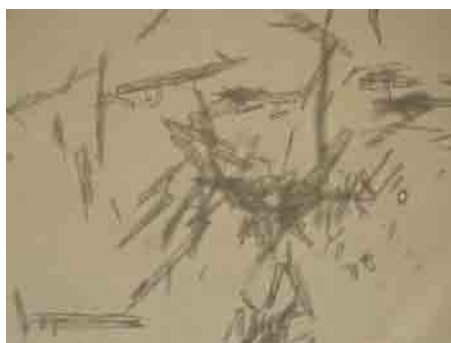
Figure 4.6 –5-ASA in its dry powder form. It is in a needle like structure.
