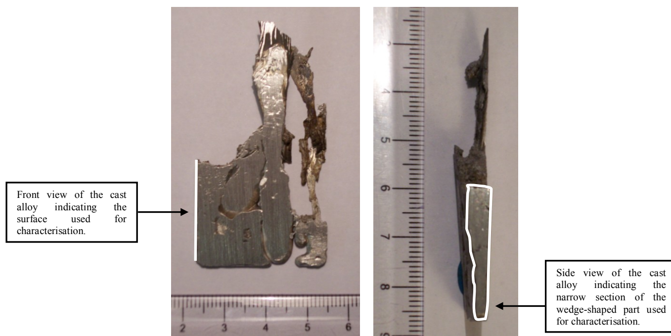
Figure 4.8 Outer surface appearance of a typical cast alloy. The cross-sectional surface used for characterisation of the alloy is shown.
