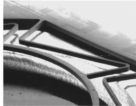
Figure 2: Each of the eight miniature legs carries three conducting wires onto the surface of the ring itself.
