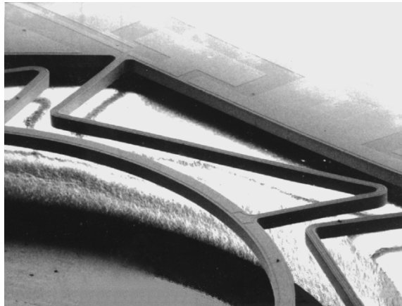
Figure 5 Microscopic View of Silicon VSG Resonator Each of the eight legs carries three conducting tracks onto the surface of the ring
