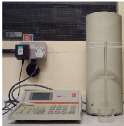
Figure 3.11: Capintec CRC-15R dose calibrator
