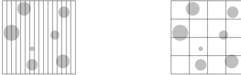
(a) Spatial decomposition in one dimension only (b) Decomposition in two dimensions simultaneously
