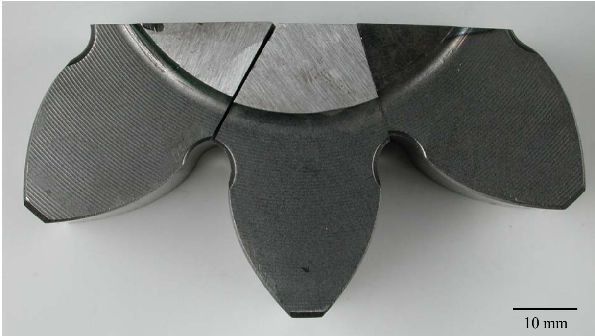
Figure 3-13 Illustration of the lower part of the steering column with the examined teeth cut from the shaft
