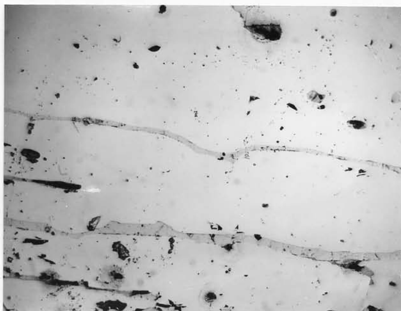
Fig. 8.5 Optical micrograph of bulk specimen SST at 1100°C, furnace cooled and aged at 600°C for 100 hours. (x 250).
