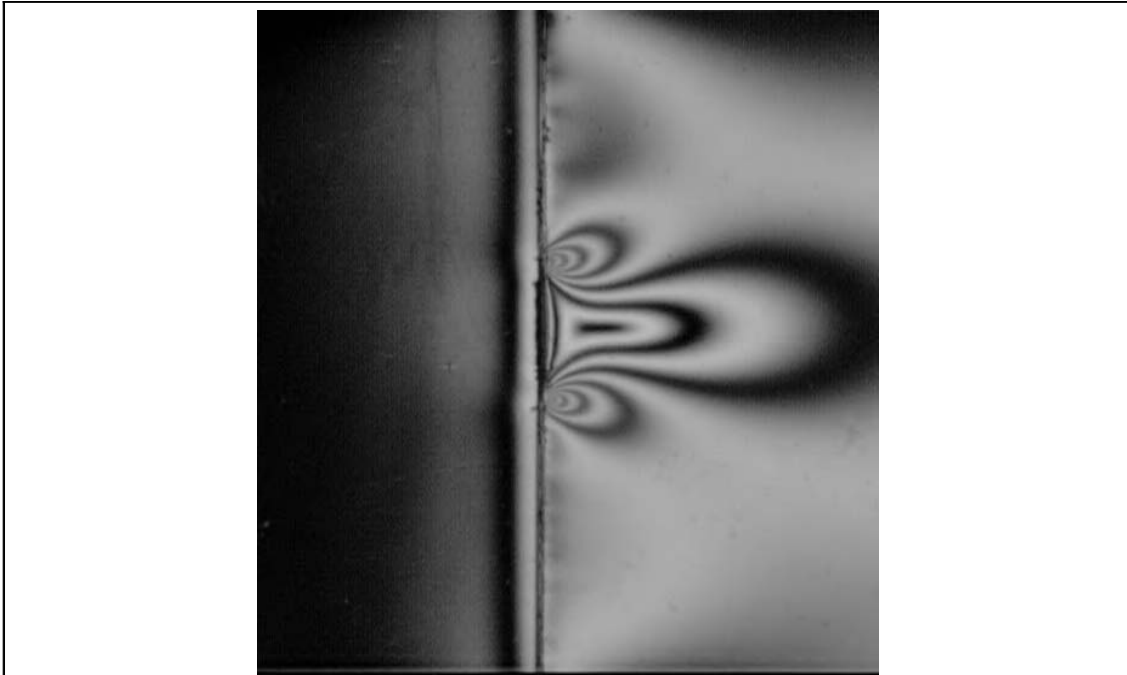
Figure 52: Isochromatic Fringe Pattern in Cracked Plate, (Source: [80])
