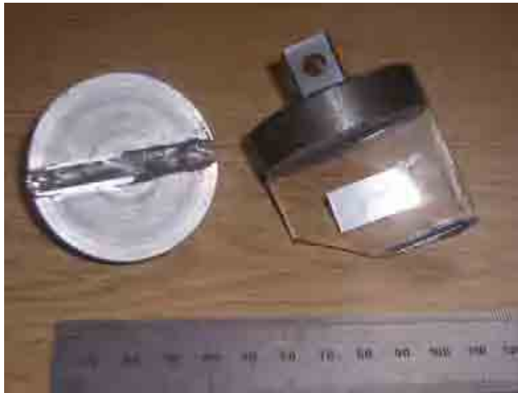
Figure 62: Failed Sample, Showing Cracking Along Interface
