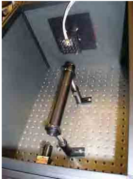
Figure 91: Laser Enclosure (25mm tapped hole pitch in bench for scale)
