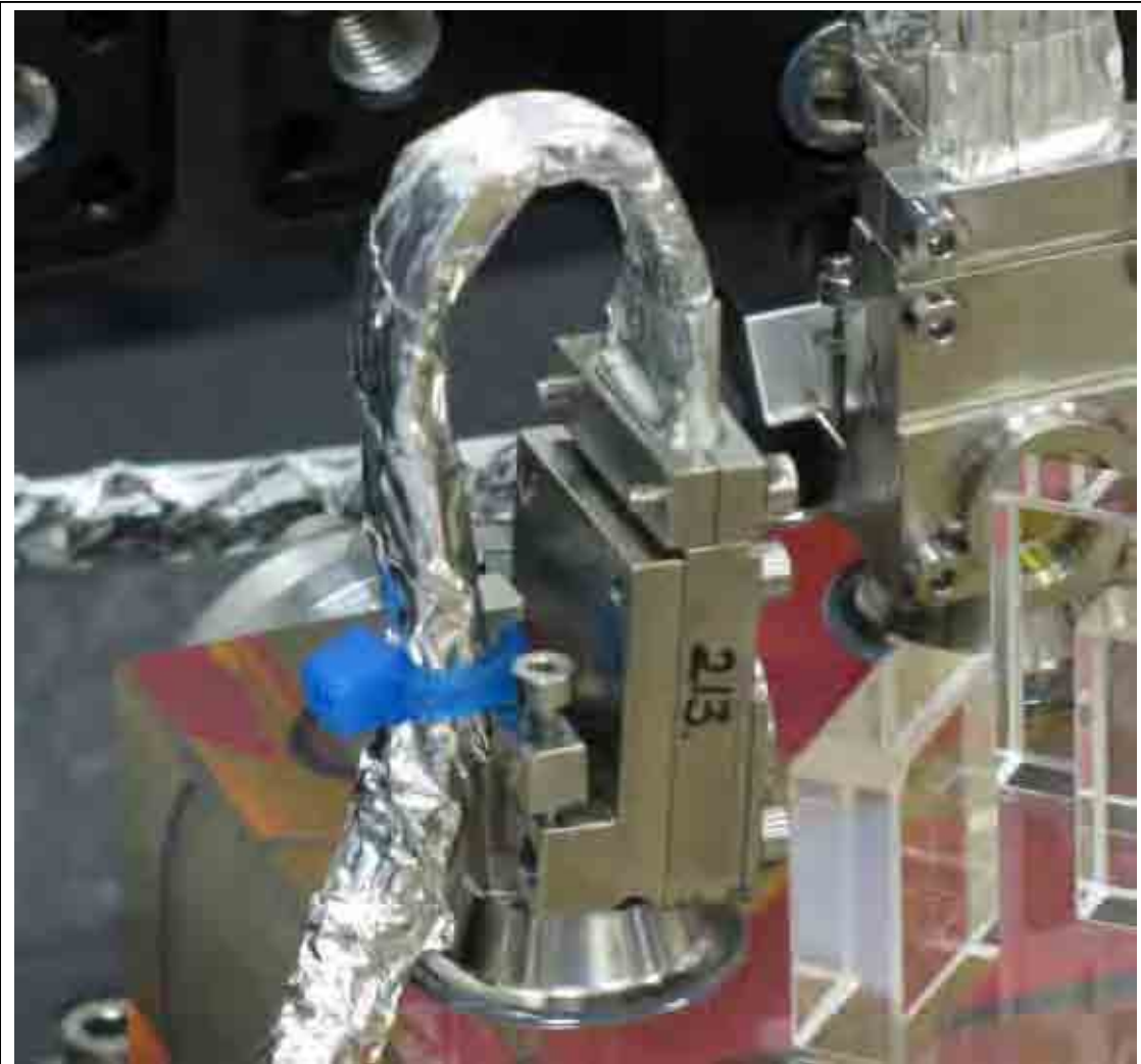
Figure 10: Photodiode Bond Detail
