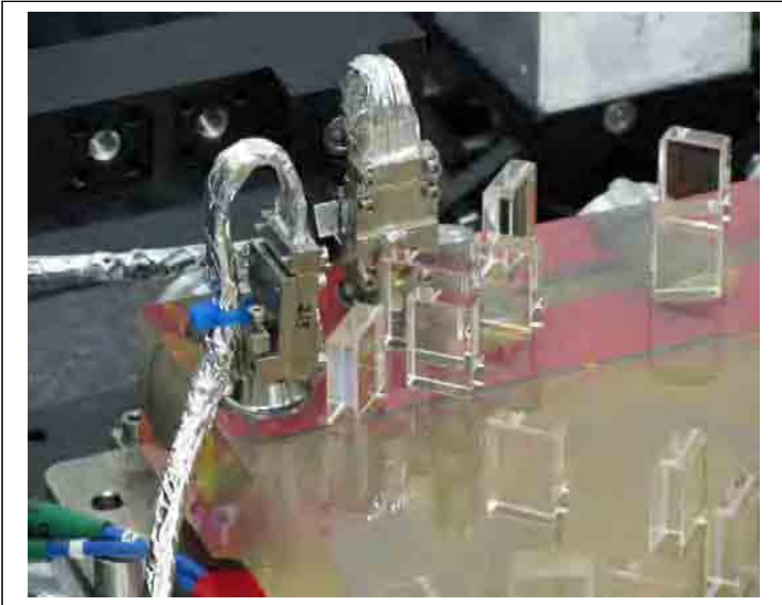
Figure 130: Photodiode PDFB Positioned from Side
